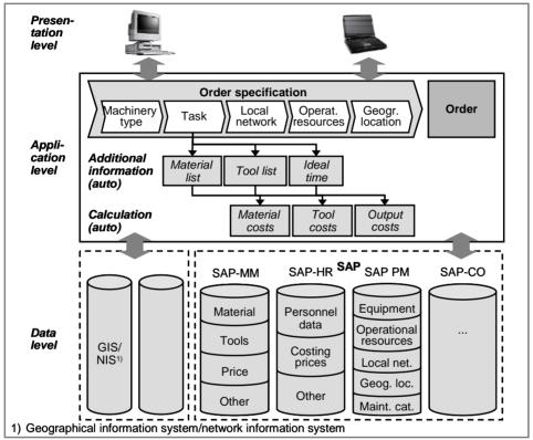
Figure 1.5: IT architecture for maintenance systems; Source: A.T. Kearney
